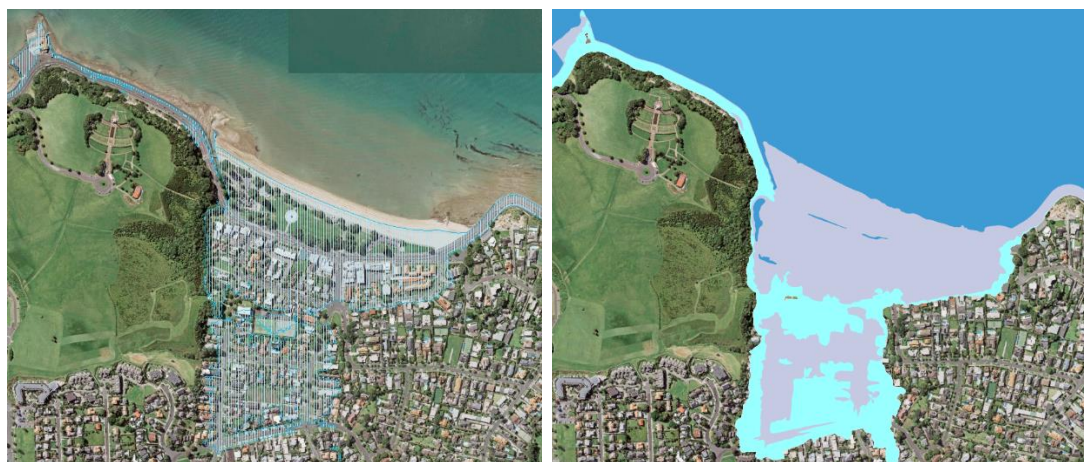
Figure A.3.2: Coastal storm inundation mapping and planning overlay at Mission Bay, Auckland
