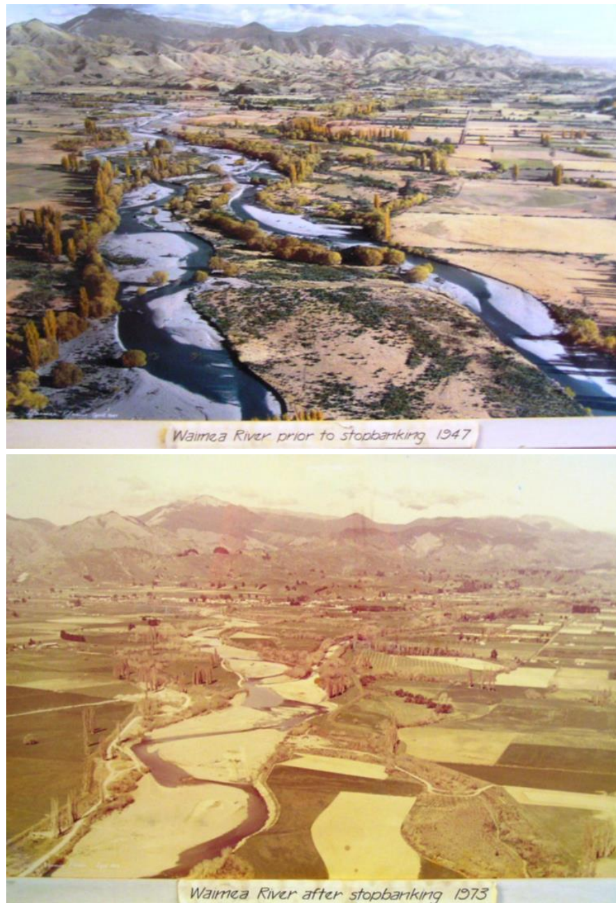
Figure 3 The Waimea River (Tasman District) before (upper, 1947) and after (lower, 1973) stopbanks were instated showing the simplification of channel form after flood protection infrastructure.
